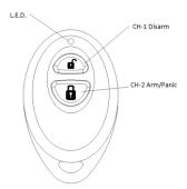
Note: To replace the batteries in the transmitter, gently to separate top and bottom cover by fingers, take out old batteries and replace with new one, ensure correct polarity.
